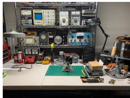
Dave is configured to service solid state armed with a multi-featured transistor analyzer (lower right blue and silver unit) combining power supply, RF generator, voltmeter, transistor tester, and current drain tester. This unit has dual power supplies supplying either 6 or 12 volts with a robust higher current setting for older car radios.
