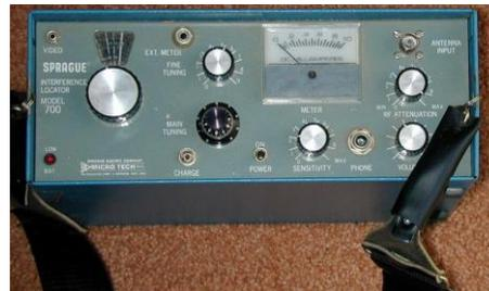
This specialized equipment enables you to monitor the symptoms as received by the customer's antenna. The setup should include a broadband AM receiver that covers the frequency range affected by the problem, an oscilloscope (scope) and an attenuator or RF gain control to adjust the RF
