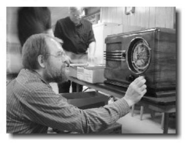
(Don't ask me to do it, though.) Jiri also demonstrated a very interesting and rare radio set. It was an Ingelen 538W. It was made in Austria in the late 1930's. It featured a unique dial that would "light" the city you were tuned into. There were 120 separate glass rods in the set in order to accomplish this feat. (All before the advent of fiber optics!) Of course, as the map of Europe changed radically every year in the late "30's, it kept the manufacturer busy updating the dial!
