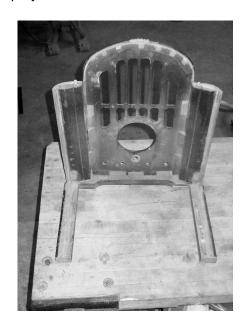
I typically dismantle severely damaged cabinets to serve as a source of cabinet repair material.
