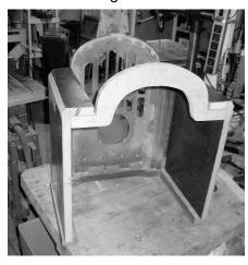
I was now faced with devising a method to form the smooth curve of the cabinet top. An attempt to bend 1/8-inch veneer plywood resulted in a splintered curve that reminded me of a porcupine in a defensive posture.
