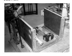
The next step consisted of sawing out the curved ends of the shoulder sections on the band saw and then using a router with an ogee bit to form the curved edge. A mortise was also cut into the bottom of the shoulder strips to accept the tenon that had been formed on the side pieces. Glue was applied to the joining areas of these shoulder pieces which were then clamped to the sides over the tenons.
