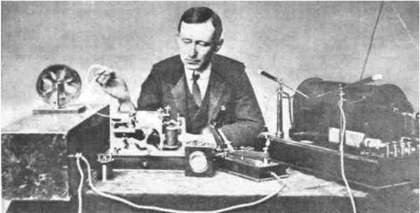
Marconi, circa 1898, with typical equipment. From right to left: 10-inch spark coil with plain gap. Key, also serving as high-voltage transmit-receive switch. Morse inker, output was to paper tape. The black box contains the secret parts: coherer and tapper, sensitive relay, and batteries.
