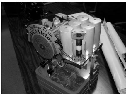
Last up was Ted Sorwika with “kit” TV that he and his brother built. The kit came with a pre-punched metal chassis and parts were bought separately. It used electrostatic deflection for the tube. It received only channel 3 - as that was the only active station when it was built. Ted said the total cost to build it was roughly \$70 (in 1947.) It was nice to see a vintage TV kit that survived all these years.
