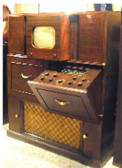
The Crosley "Swing-A-View" 12" AM/FM/Phono/TV. The CRT was pulled out and could swivel sideways for viewing at side angles.
