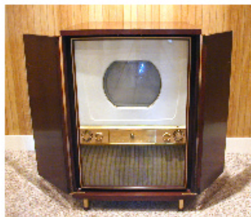
The Crosley "Swing-A-View" 12" AM/FM/Phono/TV. The CRT was pulled out and could swivel sideways for viewing at side angles.
