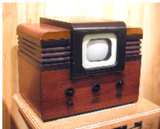
The Crosley "Swing-A-View" 12" AM/FM/Phono/TV. The CRT was pulled out and could swivel sideways for viewing at side angles.
