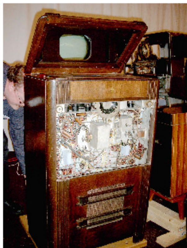
Inside view of RCA's 1934 RR-359 engineering prototype receiver. This set is restored and working.
