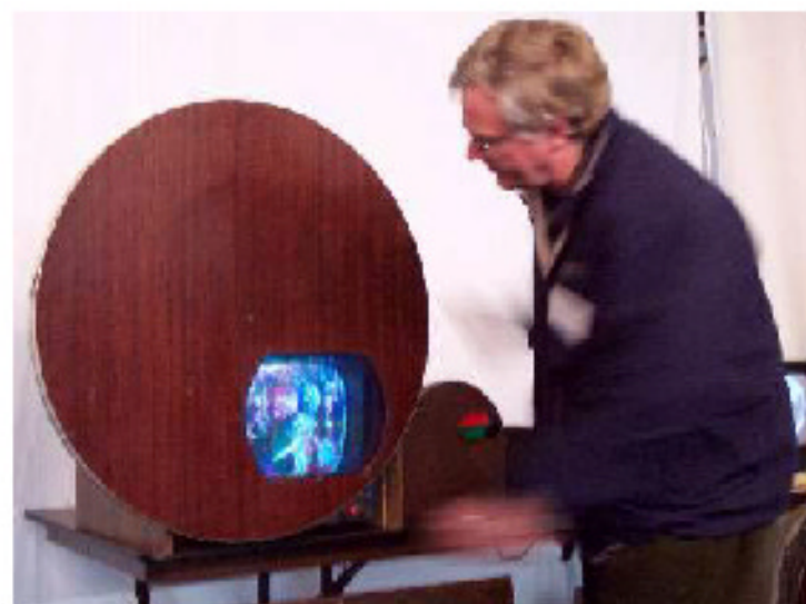
Dave Johnson displays his Col-R-Tel color converter. It was an aftermarket attachment to convert a B&W television to color via mechanical scanning.
