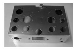
I used aluminum spray paint. As I expected, the chassis looked too shiny, so I so I rubbed it down with rottenstone, a very mild abrasive. This gave the chassis a more original, less glossy finish.
