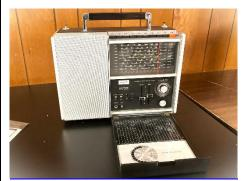
**Above:** The Lloyd's 9N24B-37A is a multiband analog radio that receives LW, AM, FM, VHF LO,
