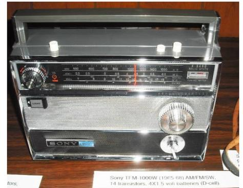
Sony TFM-1000W (1965-68) AM/FM/SW. 14 transistors, 4X1.5 volt batteries (D-cell) for.
