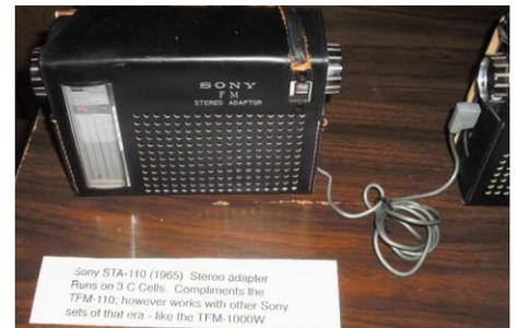
Sony STA-110 (1965) Stereo adaptor. Runs on 3 C-Cells. Complements the TFM-110; however works with other Sony sets of that era - like the TFM-1000W
