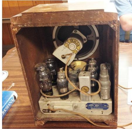
**Above:** Jiri Placek showed a Delco 3201 farm set which employs a robust pair of push-pull 48's in its audio circuit. It was ready to utilize the standard 32 volt DC system often used on farms and also manufactured by Delco **shown below**.
