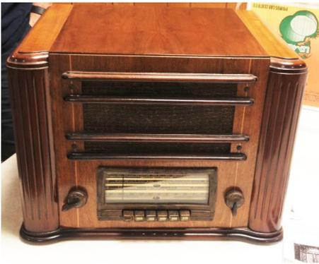
**Above:** Tom Lager showed a 1940 Silvertone 6359 which was value-priced at \$29 to \$35 including the A&B batteries. This was a 6 tube 4 band set employing 1.5 volt tubes and a class B amplifier circuit with AVC. Tom totally refurbished the cabinet and chassis of this beautiful radio.
