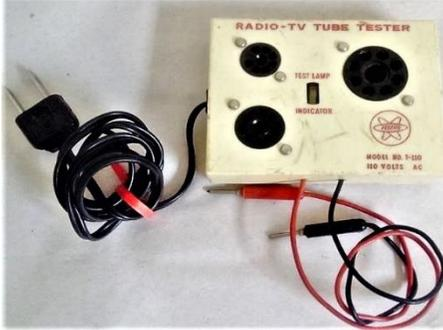
**Above:** Al Simmons shows compact tube tester, the T-110 from the great folks at Fedtro, purveyor of many money saving (read cheap) devices. Why waste your time carrying your tubes to the drug store when you can test any tube with this unit priced under \$10? But it does test for filament continuity with a neon lamp indicator. Al showed some other bargain offerings from Fedtro.
