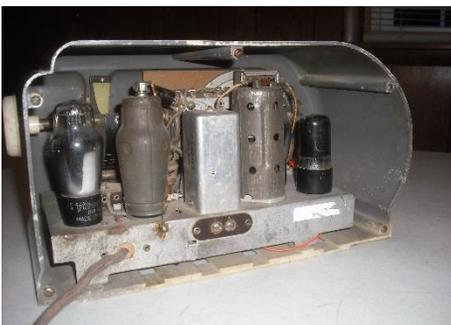
**Below:** Jiri Placek demonstrated a project to restore a damaged Plaskon Cabinet. More amenable to epoxies since more flexible to the drilling than Bakelite due to processing without first grinding into powder, these Plaskon fix operations can be accomplished with supplies like epoxy resin, T-nuts, a good drill, ash black from printer cartridge for tinting, crazy glue, sand paper and auto polishing compounds.
