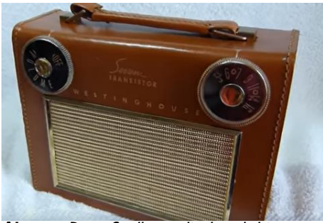
Above: Dave Snellman displayed this Westinghouse H602P7 lovingly restored by NJARC member Charles Blanding. Made in Metuchen, NJ, this 7 transistor was Westinghouse's first solid state radio offering. https://www.youtube.com/watch?v=f59b9S7SaIA
