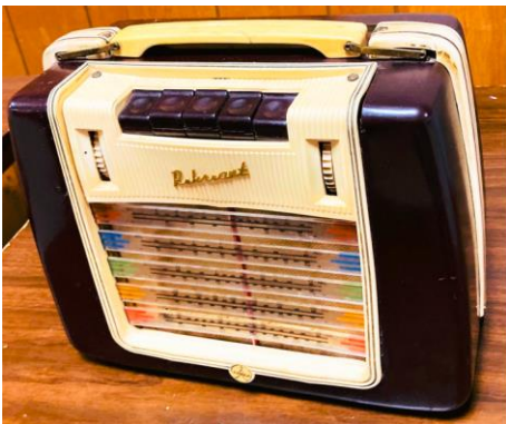
Below: Jiri Placek showed a Tesla Rekreant 3103 AB from 1957 manufactured by Tesla in Czechoslovakia. The slide rule tuning covers 5 bands for ranges of Long Wave, Broadcast and Short Wave and is very colorful. Rekreant translates to Vacationer as this radio can run on batteries 90 + 1.5 V or on house current. Instead of a telescoping antenna, it uses 4 dedicated loop antennas for various bands. Color codes on the pushbuttons translate to the band color below. Tesla was basically a cartel formed to nationalize manufacturers such as Telefunken, Siemens and 14 more manufacturers and the name Tesla was a nod to but not started by Tesla himself. Tesla instituted price controls, protections, but after the Soviet dissolution could not compete with Asian products.
