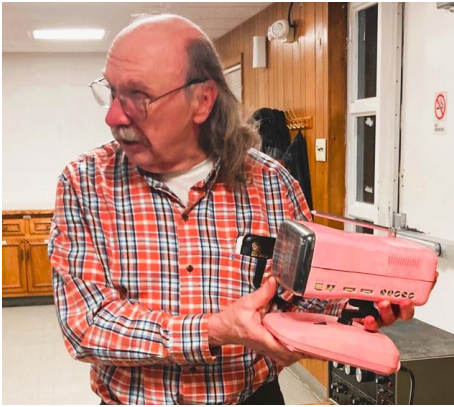
Below: Jiri Placek showed a Tesla Rekreant 3103 AB from 1957 manufactured by Tesla in Czechoslovakia. The slide rule tuning covers 5 bands for ranges of Long Wave, Broadcast and Short Wave and is very colorful. Rekreant translates to Vacationer as this radio can run on batteries 90 + 1.5 V or on house current. Instead of a telescoping antenna, it uses 4 dedicated loop antennas for various bands. Color codes on the pushbuttons translate to the band color below. Tesla was basically a cartel formed to nationalize manufacturers such as Telefunken, Siemens and 14 more manufacturers and the name Tesla was a nod to but not started by Tesla himself. Tesla instituted price controls, protections, but after the Soviet dissolution could not compete with Asian products.
