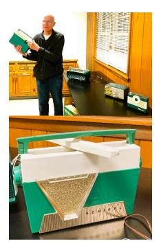
**Below:** Here is a two-tone Hallicrafters 612 from 1954 with an RF preselector stage using an additional 12BA6.
