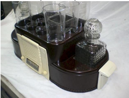
Above and Below: A S-W 07-5B, a 4-tube superhet with regeneration. Some of these "Senior Varsity models" could be acquired in a college theme, usually with a letter in school color on the grill. Be true to your school!
