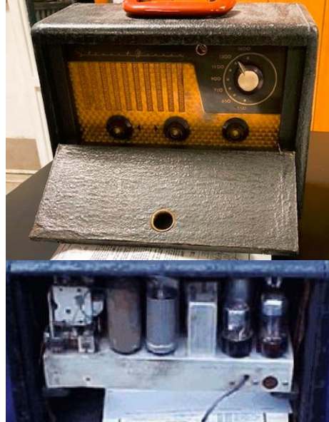
1A7GT 1N5GT 1H5GT 3Q5GT 3S25GT 3S25GT Battery Pack, Eveready 753, Ray-O-Vac AB-994, Burgess F6A60, General 60A-6F6-5
