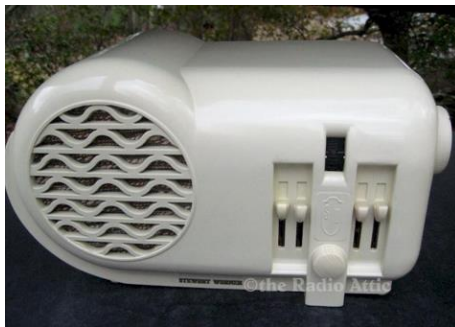
Above and Below: A S-W 07-5B, a 4-tube superhet with regeneration. Some of these "Senior Varsity models" could be acquired in a college theme, usually with a letter in school color on the grill. Be true to your school!
