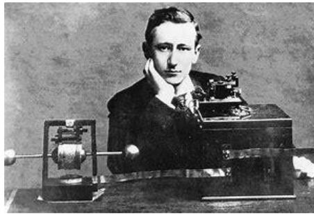
Illustrated in a radio book was an induction-coil "Experimental Wireless Set." The 1909 edition of *Operator's Wireless Telegraph and Telephone Handbook*, still on my bookshelf, showed how to do it. With no tuned circuits, you hooked an antenna to one side of the spark gap, the other side to ground, just like in the picture, simple as that.
