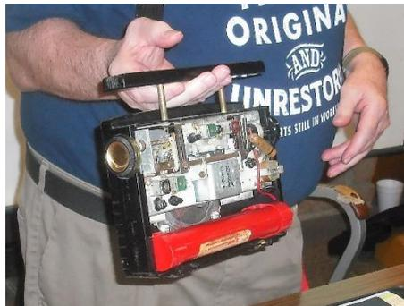
**Above:** Dave is grabbing the ingenious spring-loaded handle of a Zenith Royal 800. The handle enclosed the antenna of this 1957 model which used point to point wiring with transistors. **Below:** On a Zenith note, Dave showed one of the first hearing aids which included zenith mini-tubes and went through batteries rapidly. Zenith's visionary co-founder and CEO, Commander E. F. McDonald may have suffered from hearing impairment leading to interest in hearing aid development.
